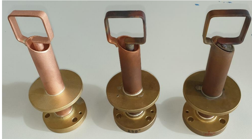
(from left to right: loop in original condition; strongly warmed loop; irreparable loop)
