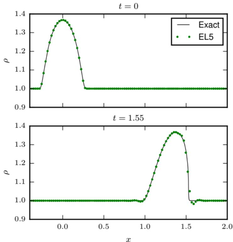
A non-linear, smooth hydrodynamical wave, propagating to the right and tilting in the direction of its motion, until a caustic is produced.
