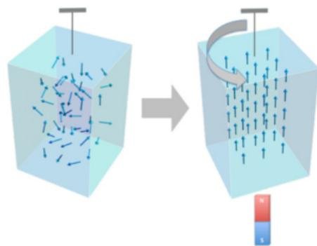
**Figure:** Application of magnetic field on an unmagnetized metallic object induces magnetization, body start rotating (mechanical angular momentum emerges)
