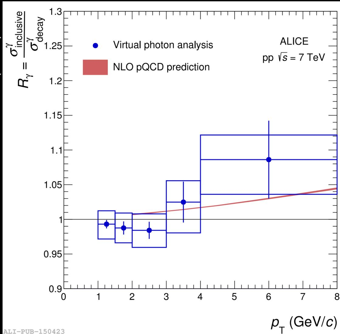
Real and virtual-photon yield connected by the Kroll-Wada equation ( $p_{T,ee} > m_{ee}$ )
